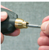
Fig. 3: Place retracted BRUSH on pins and twist
