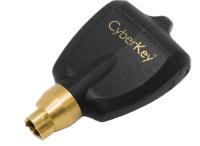
The CyberKey is an electronic key used to operate CyberLock cylinders. It has memory that contains encrypted access codes, a list of locks it may access, schedules of authorized dates and times it may access locks, and a begin-end date range during which the key will operate. The battery from a CyberKey energizes the electronics within a CyberLock cylinder.
