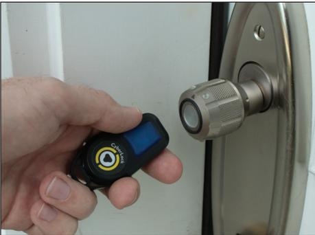
Open FlashLock using an infrared key fob.
